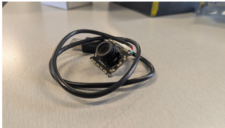
Figure 5. The repurposed webcam module used to capture light-intensity changes from the finger.
