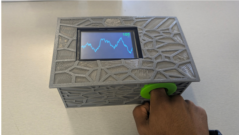
Figure 18. The completed enclosure with the screen operating and flexible finger interface in use.
