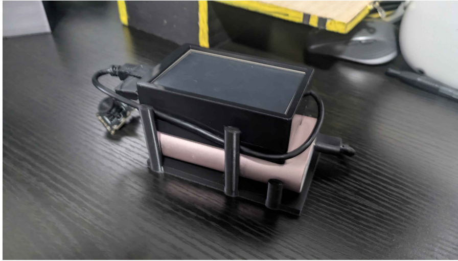
Figure 12. The final internal chassis with the shorter and more flexible black micro-USB cable.
